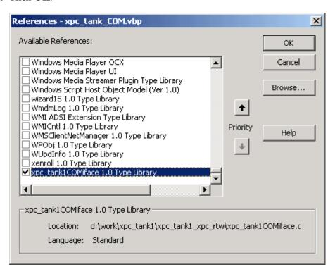
The model-specific COM API Type Library (xpc tank1COMiface.dll) is now available for use in your project. Sections "Viewing Model-Specific COM Signal Object Classes" on page 4-25 and "Viewing Model-Specific COM Parameter Object Classes" on page 4-26 describe how to look at class objects.
